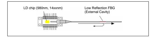
Pump LD wavelength stabilizer is used for external cavity of pump Laser Diode. 980nm and 1420-1490nm wavelength ranges are available.
