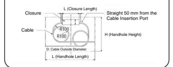
The cable entry section is in-line, making it ideal for use in space-constrained manholes and handholes.
