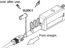
Be careful not to slant SC connector while inserting into the Guide cap.
