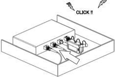
Be careful not to slant the One-Click<sup>TM</sup> Cleaner SC Mini while inserting into the adapter.
