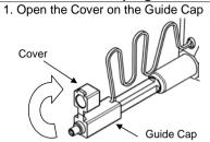
2. Insert MU/LC connector into the Guide Cap
