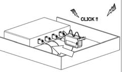
Be careful not to slant the One-Click<sup>TM</sup> Cleaner MU/LC Mini while inserting into the adapter.
