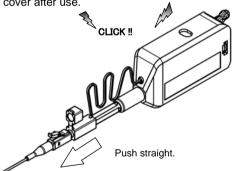
Be careful not to slant MU/LC connector while inserting into the Guide cap.
