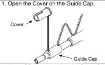
Insert SC connector into the Guide Cap.
