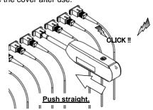
Be careful not to slant the One-Click<sup>TM</sup> Ultra Cleaner 2.5 while inserting into the adapter.
