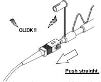
Be careful not to slant connector while inserting into the Guide cap.
