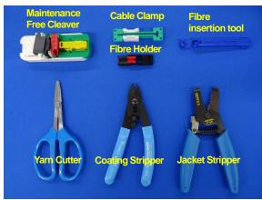
Note: Maintenance Free Cleaver Green for SM fibre Blue for MM fibre
