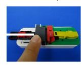
Press down the black unit to engage the blade, while keeping fibre holder stable
