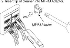
3. Push the Outer Shell to start cleaning the MT-RJ connector end face. An audible "click" sound indicates end of cleaning process. Close the cover after use.
