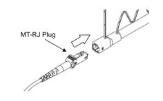
3. Push the Outer Shell to initiate the cleaning the MT-RJ connector end face. An audible "click" sound indicates end of cleaning process. Close the cover after use.
