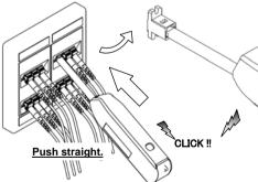
Be careful not to slant the One-Click<sup>™</sup> Cleaner MT-RJ while inserting into the adapter.
