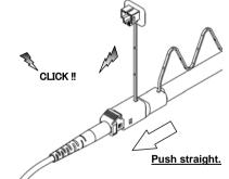
Be careful not to slant connector while inserting into the Guide cap.
