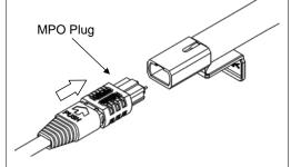
3. Push the Outer Shell to initiate the cleaning the MPO connector end face. An audible "click" sound indicates end of cleaning process.
