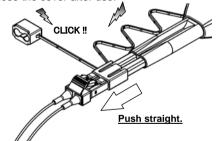
Be careful not to slant connector while inserting into the Guide cap.
