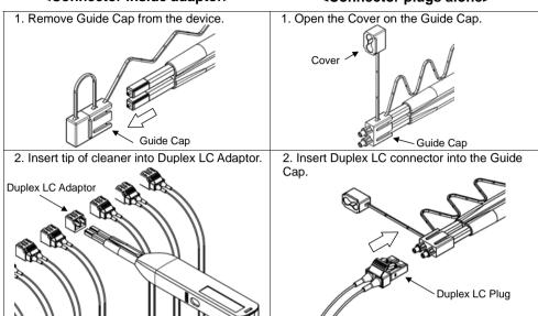
3. Push the Outer Shell to start cleaning the Duplex LC connector end face. An audible "click" sound indicates end of cleaning process. Close the cover after use.
