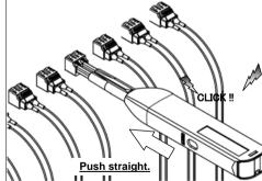
Be careful not to slant the One-Click Cleaner D-LC while inserting into the adapter.
