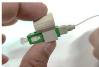
2. Insert the cleaved fiber into the connector
