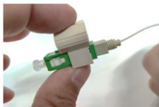
2. Insert the cleaved fiber into the connector
