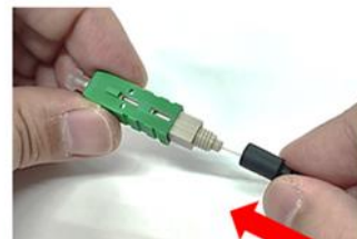
4. Lastly, push the boot onto the connector's body
