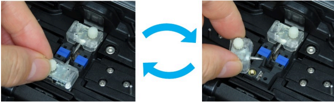
Electrode replacement without tools
